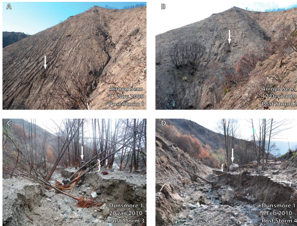
Figure 5. Paired photographs of post-event erosion at (a and b) Arroyo Seco and (c and d) Dunsmore 1. The hillslope and channel erosion characteristics shown in the photographs are representative of the erosion we observed at the other study sites. Photos were taken on the dates listed in the figure, which were less than one week after a debris-flow. Common reference points in the two pairs of photos are shown with the white arrows. In Figure 5a hillslope rilling was very pronounced after the first storm and debris flow at Arroyo Seco. Post-event dry ravel can be seen beginning to refill the steep channel. In Figure 5b the second storm at Arroyo Seco substantially eroded the well-developed rill network shown in Figure 5a. Figures 5c and 5d show channel erosion 290 m downstream of the Dunsmore 1 station (upstream area = 1.45 km 2 ) caused by the 18 January 2010 and 6 February 2010 debris flows. The white brackets in Figures 5c and 5d show the height of a person standing in the photos.
