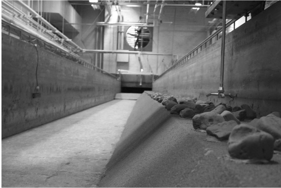
Fig. 2. View looking up the USDA-NSL 100 ft flume. The acoustic Doppler current velocimeter is shown on the right side of picture. The width of the flume including the floodplain is 1.22 m.
