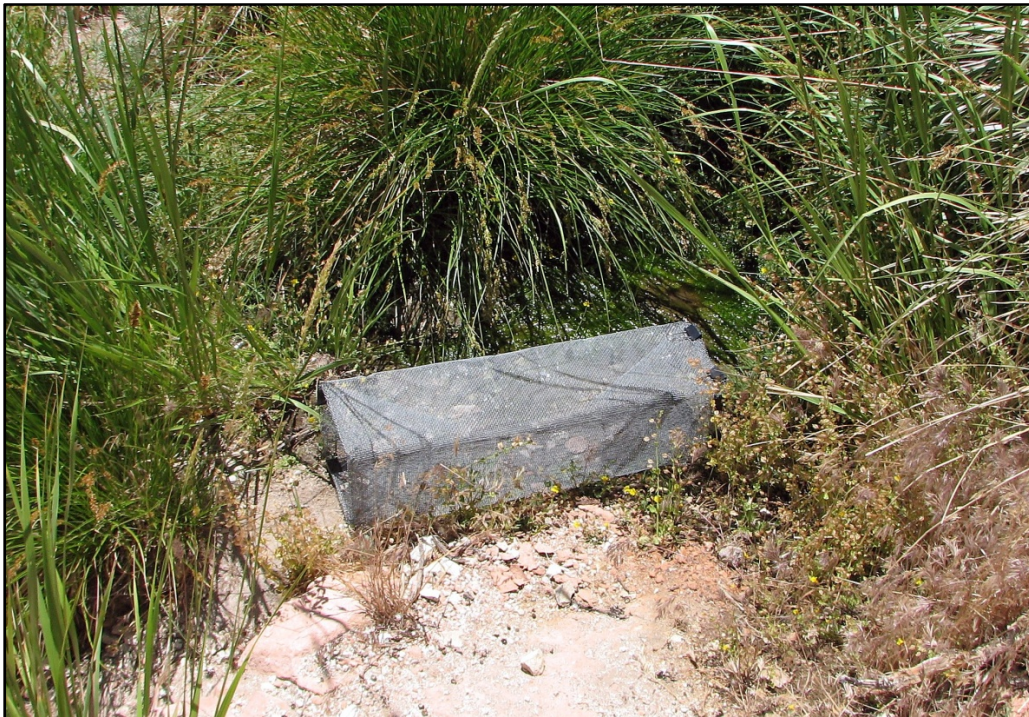
Figure 6-4. Rectangular wire-mesh funnel trap (Photo by D. B. Hall, June 2, 2009)
