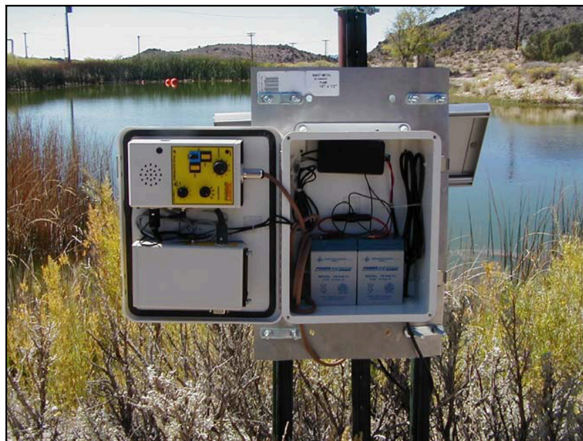
Figure 6-24. Passive acoustic monitoring system at Camp 17 Pond. (Photo by D. B. Hall, September 23, 2003)
