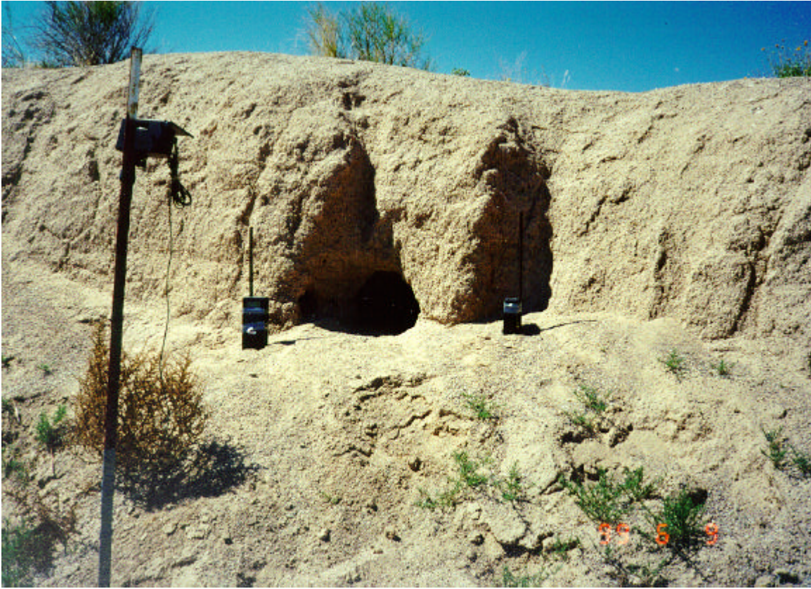
Figure 6. TM 1500 still camera system set up at an owl burrow (transmitter on right, receiver on left)
