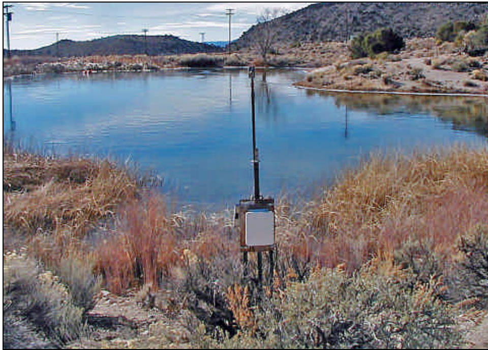
Figure 5-11. Passive acoustic monitoring system at Camp 17 Pond. (Photo taken by Derek Hall on November 30, 2004.)
