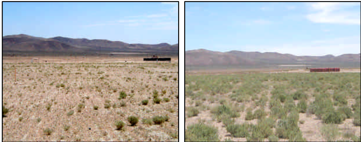
Figure 6-8. Comparison of vegetative cover, growth, and establishment on CAU 110, U-3ax/bl closure cover. Photos were taken by Dave Anderson in June 2003 (left) and June 2005 (right).
