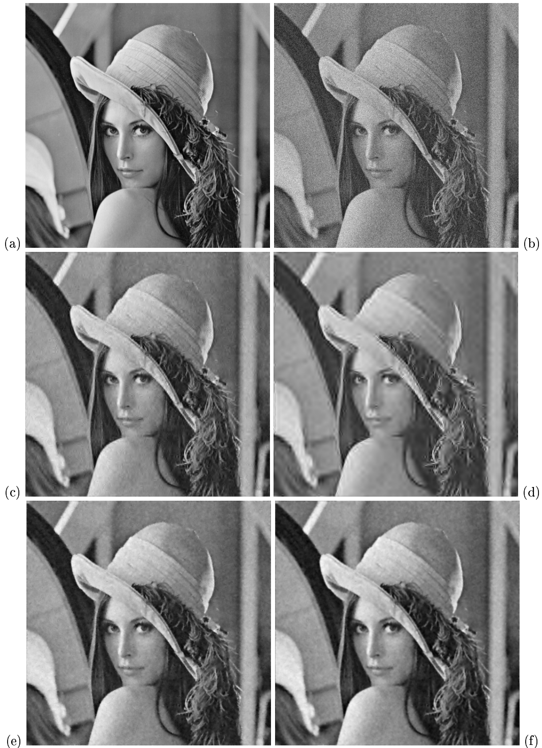
Figure 3: Denoising results for the Lena image. (a) Original image. (b) Noisy image, \sigma = 20 , MSE = 399.50 . (c) SureShrink , MSE = 61.59 . (d) Global universal rule with hard thresholding, MSE = 103.95 . (e) Minimum mean squared error ( 5 \times 5 ) followed by Gaussian ( 3 \times 3 ) filter, MSE = 56.80 . (f) Minimum mean squared error ( 5 \times 5 ) followed by mean ( 3 \times 3 ) filter, MSE = 64.80 .
