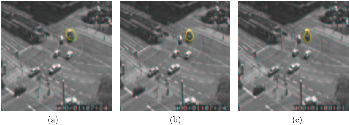
Figure 1: Evolution of the Chan-Vese segmentation contour: initial contour (a), an intermediate contour (b), and final contour (c).
