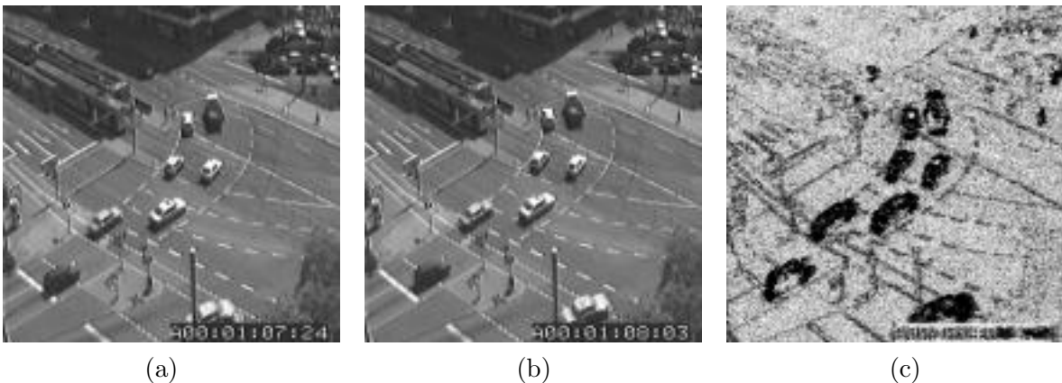
Figure 3: Two frames of a video (a), (b), which are approximately 1/5 second apart, and their difference (c).
