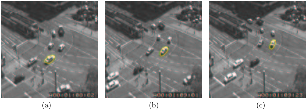
Figure 2: Results of the Chan-Vese-based tracking algorithm over time. Each frame of video was used in tracking the object and the results are shown at approximately one second intervals.
