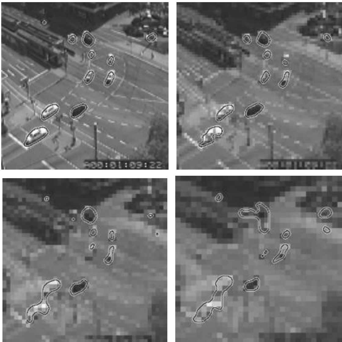
Figure 10: Segmentation of Figure 9(c), where the spatial resolution has been reduced 16x (a), 64x (b), 144x (c), and 256x (d).
