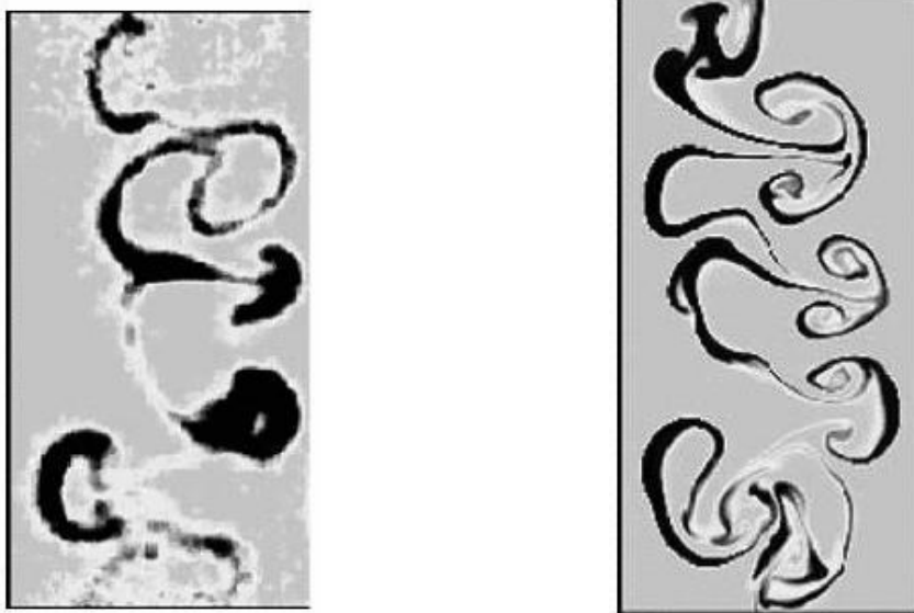
Figure 1: The left image shows the von Kármán vortex pattern of a Richtmyer-Meshkov experiment performed at Los Alamos National Laboratory. The same experiment is simulated by high resolution numerical methods and the result is shown in the right image [Rider et al., 2002].
