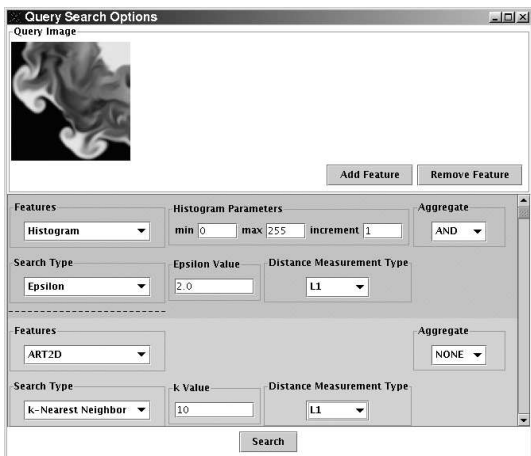
Figure 4: This figure illustrates how a similarity search is defined. The top left image is the query image specified in Figure 3. Two features, “Histogram” and “ART2D”, are used in this search, and their respective search parameters are specified in the two rectangular regions shaded in different gray levels.
