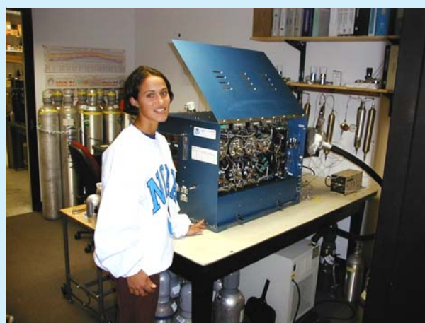
A 12-compound gas chromatograph developed and built by CMDL for operation at the baseline stations.
