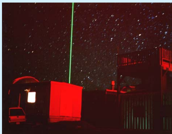
Mauna Loa stratospheric aerosol lidar in operation at night. The vertical green streak is the laser beam.
