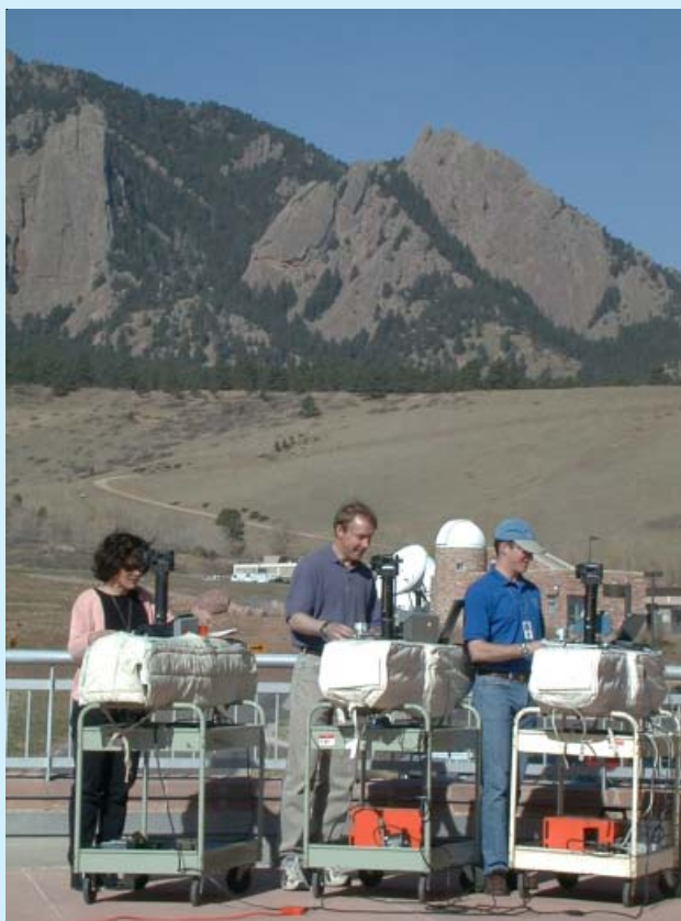
Dobson ozone spectrophotometer calibration.
