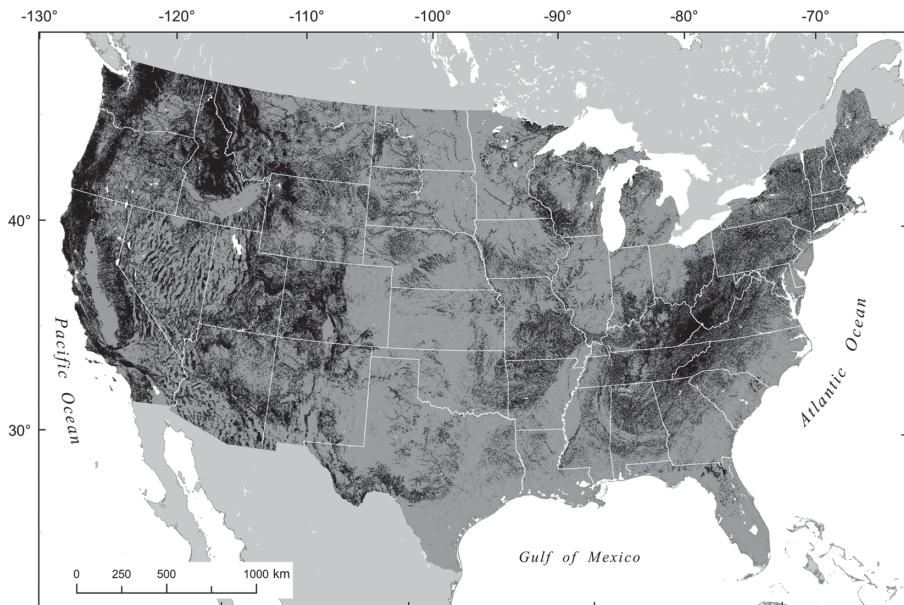
Figure 3. Prototype map showing areas of the conterminous U.S. with negligible (gray) and some (black) susceptibility to landslides.
