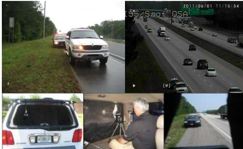
Figure 10: In a study on compliance with Move Over laws and the effects of emergency lighting on compliance, the Florida Highway Patrol placed a patrol car and research vehicle at the roadside to simulate a traffic stop and recorded the speed and lane behavior of passing vehicles (Photos: Florida Highway Patrol and Florida Department of Transportation).
