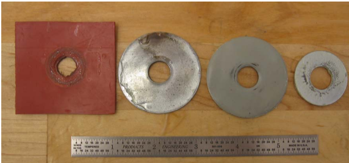
Figure 2-6: Various isolation washers, from left to right, rubber washer, fender washer with epoxy coating, fender washer with JB weld epoxy coating, conventional 1/2" washer with epoxy coating.
