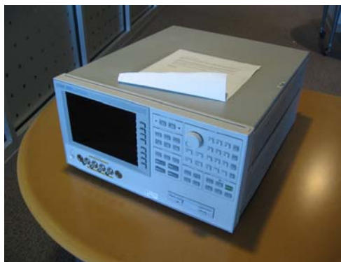
Figure 3-1: Agilent 4294A impedance analyzer, $41K
