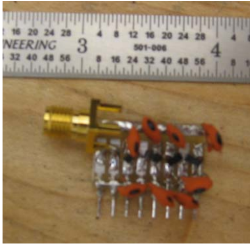
Figure 4-4: 8X Voltage Rectifier
