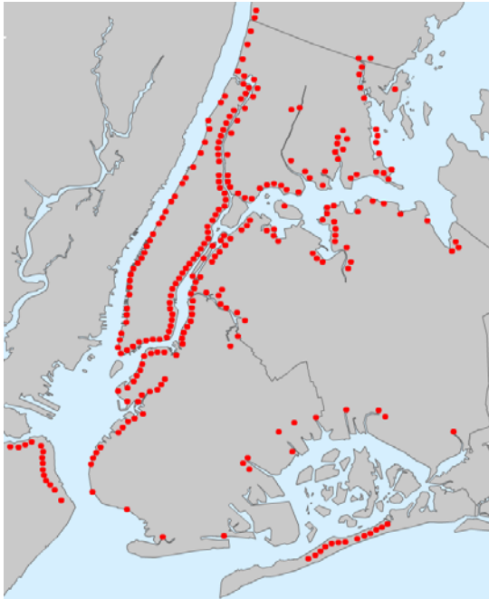
This map of New York Harbor shows the locations of some of the 460 CSOs citywide, indicated by red dots. Image: Sustainable South Bronx. For a more detailed map, see http://www.nyc.gov/html/dep/pdf/hsurvey97.pdf
