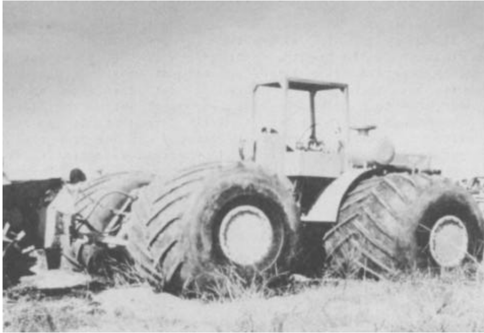
Figure 5-15. Rubber-tired rotary trencher
