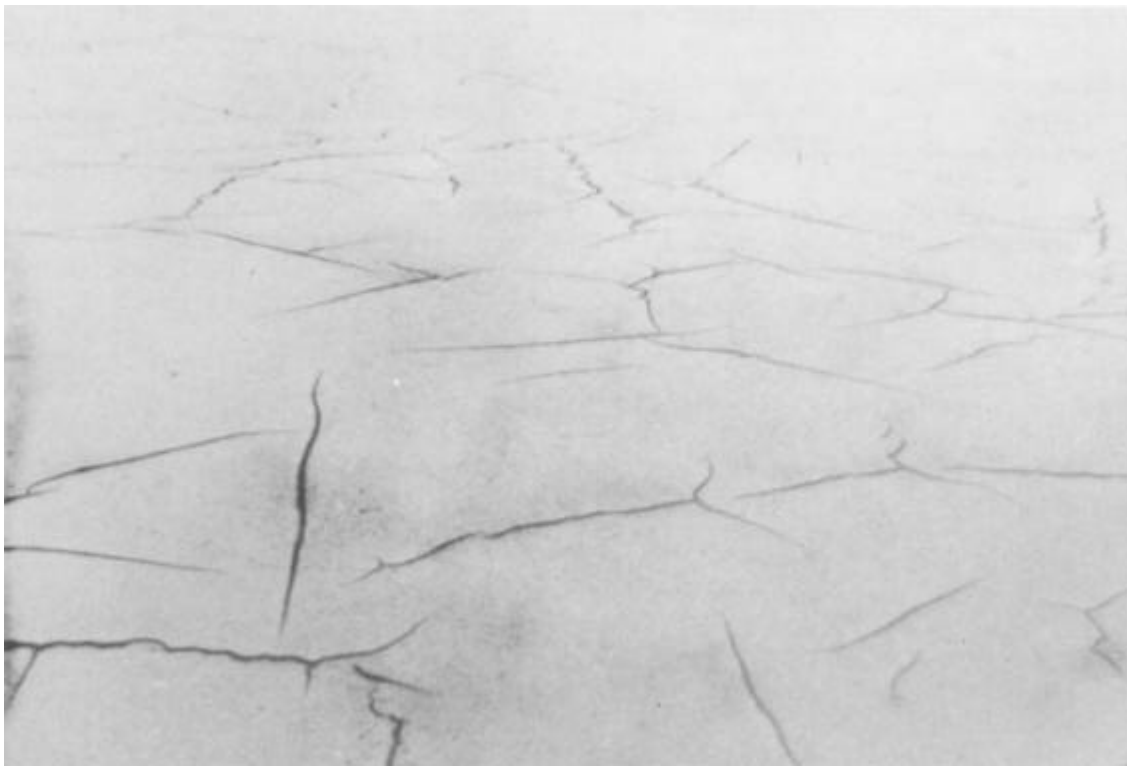
Figure 5-8. Surface of fine-grained dredged material at the earliest time when surface trenching should be attempted; initial cracks are spaced at 3- to 6-foot intervals, and the surface water content approaches 1.8 \times LL
