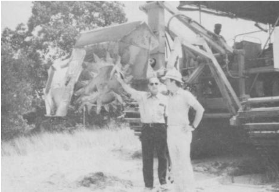
Figure 5-17. View of hemispherical rotary trenching implement
