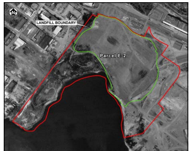
1974 Aerial Photograph. Landfill covered with soil (between 2 and 5 feet thick).
