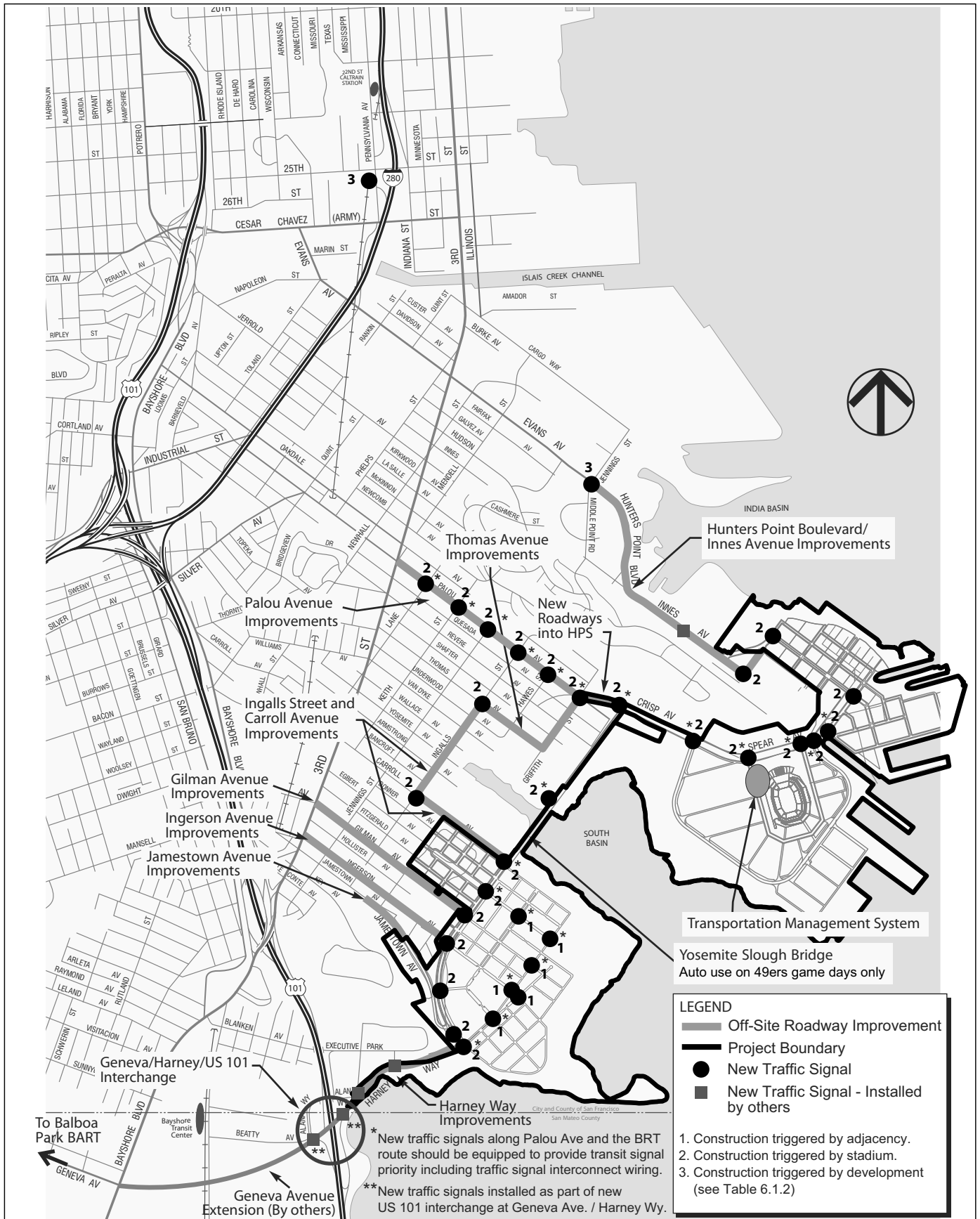
Candlestick Point Development Traffic Signal Improvements
