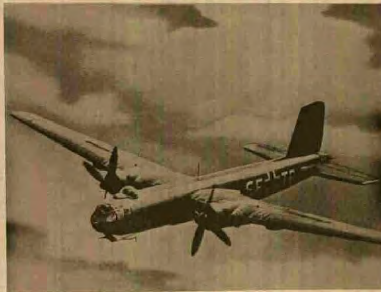
Figure 6 Germany's "ugly duckling," the Heinkel He-177 heavy bomber. Two engines were placed side by side under a single nacelle, giving this four-engine plane the appearance of a twin-engine bomber
