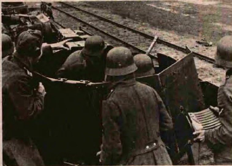
Figure 37 Flak gun (2-cm.) going into action aboard an armored train
