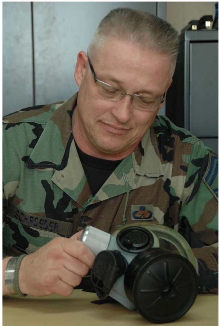
Senior Master Sgt. Scott Schroeder uses his invention to easily remove and replace the D-ring voice-mitter in the gas mask.
