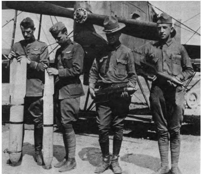
Four different types and sizes of bombs used in raids: (l. to r.) 155-mm, 115-mm, 90-mm, and 75-mm.
