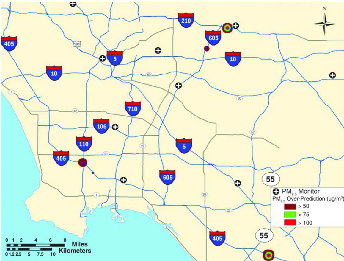
Figure 13. Map of over-predicted values from the LUR model, shown as > 50 , 75 , or 100 \mu\text{g}/\text{m}^3 higher than the measured value. Most over-predictions occurred at freeway intersections. \text{PM}_{2.5} monitor positions are marked with a +.
