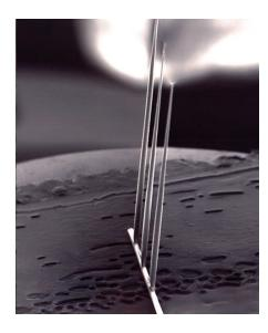
A new method for fabricating microelectronics, Lasonix can be used to form standard semiconductor microcircuits in vertical arrays, conductive interconnects, and hybrid integrated circuits in three dimensions. Shown are potential electric field emitters for microvacuum electronic devices.
