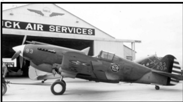
P-40 of the 55 th Pursuit Squadron at Oakland Municipal Airport in 1940. This is not a B model, but just a P-40. No production A models were made. B models had the star insignia on the fuselage and no tail stripes. This model P-40 sports two .50 cal. machine guns in the nose and one .30 machine gun in each wing. Photo from Bill Larkins
