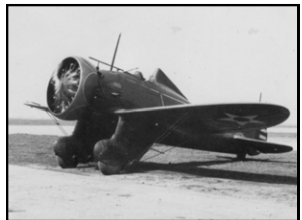
P-26A of the 77 th Pursuit Squadron. 20 th Pursuit Group P-26 aircraft did not have squadron markings. To identify them the cowl ring had a red scallop with a white strip and the engine face was also red. Similar paint scheme would be used for the 55 th and 79 th squadrons with their respective colors. Also note the long tube in front of the windscreen. This was the telescopic gun sight. The aircraft was armed with a pair of .30 caliber machine guns firing through the prop from below the fuselage.
