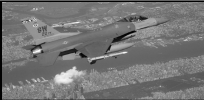
20 FW F-16CJ wing flag ship performing NORAD Operation Noble Eagle mission over New York City, NY on 24 September 2003. Armed with AIM-120C (AMRAM) and AIM-9 Sidewinder missiles, and equipped with 370-gal fuel tanks. Central Park is visible below the aircraft.
