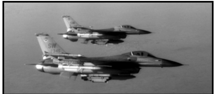
77 & 78 FS F-16s on patrol 7 April 1998 near the Iraqi border as part of Operation Southern Watch. They are carrying Low Altitude Navigation and Targeting Infrared for Night (LATNTIRN) systems and are fitted with AIM-9 Sidewinder, AGM-88 Harm (mid-wing) and AIM-120 AMRAAM Slammer missiles on the wing tips. USAF Photo
