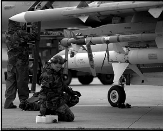
SSgt Rob Anson replaces the argon bottle in an AIM-9 missile on 19 April 1999. Anson is deployed with the 78 EFS to Aviano AB, Italy in support of Operation Allied Force.
