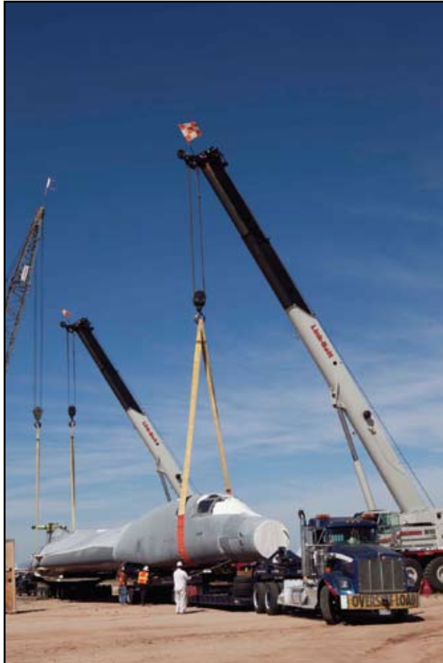
Above, AMARG crane operators place B-1B, Serial No. 85-0082 onto a customized trucking platform designed to cradle and protect the aircraft from stress during the lengthy roadtrip to Washington. Right, aircraft is sealed and protected from weather and road hazards before finally rolling out of AMARG (below).
