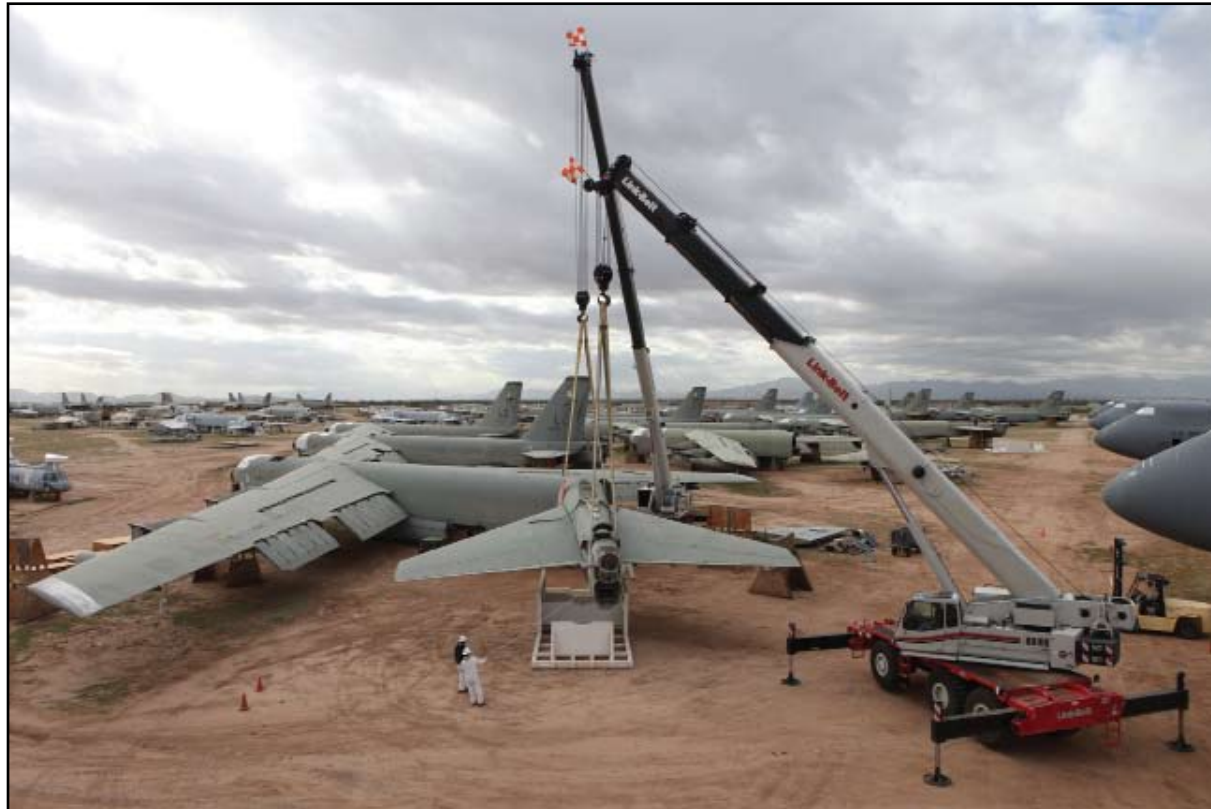
Above, AMARG crane operators lift and gently place the eliminated B-52G aft section onto a custom-built module to facilitate verification of the cut by NTM or national technical means as stipulated by the New Strategic Arms Reduction Treaty (START) protocol.
