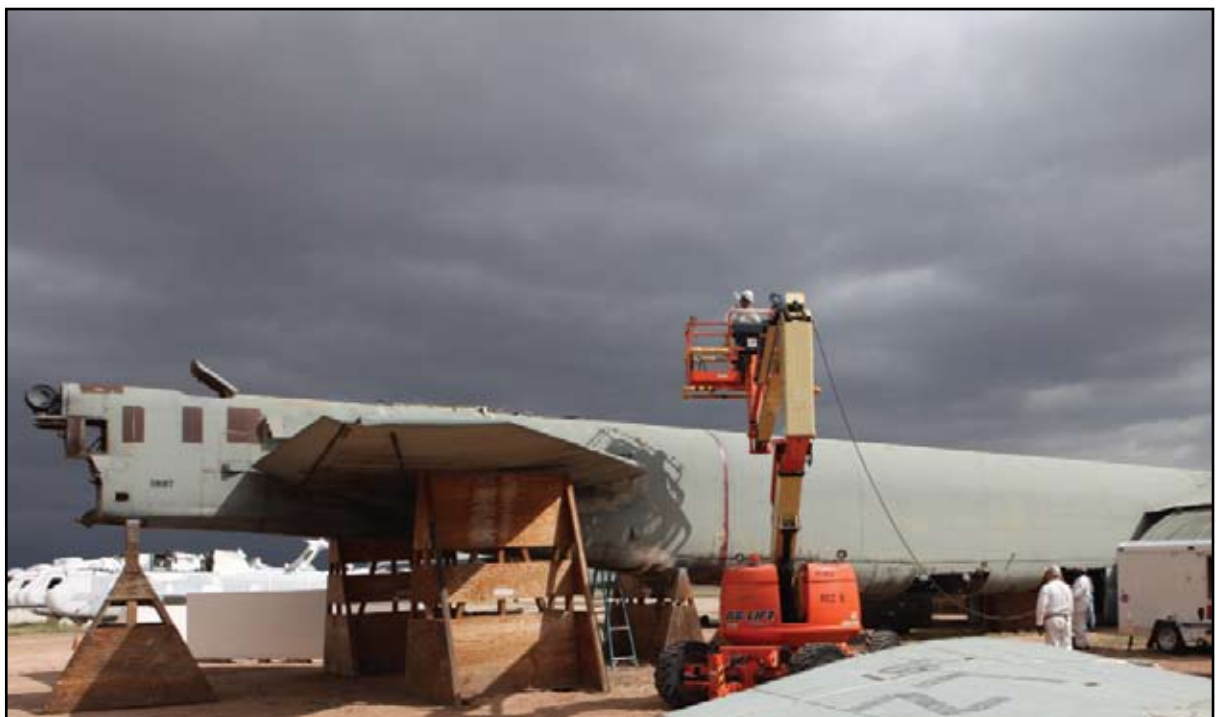
Left, AMARG’s 577th Commodities and Reclamation Squadron (577 CMRS) employees, Mr. Rodney Vakoc and Mr. Ryan Graves (cutting) make a surgical cut through the fuselage of B-52G, Serial No. 58-0197, in order to eliminate the aircraft in compliance with the New START. Below, 577 CMRS employees position themselves along the indicated cutline drawn between the airframe’s manufacturing or production breaks.
