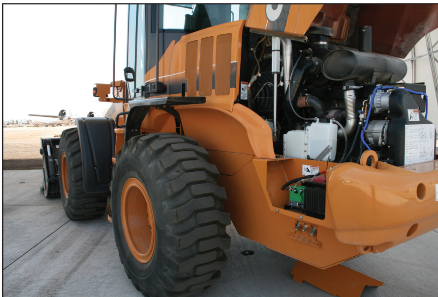
A hydrogen generator (green box situated in battery compartment) was installed on this front end loader to reduce both fuel consumption and emissions.
