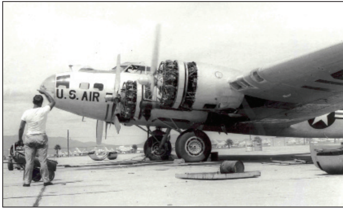
Then...a mechanic performs an engine run on a B-17 bomber in preparation for flight.
