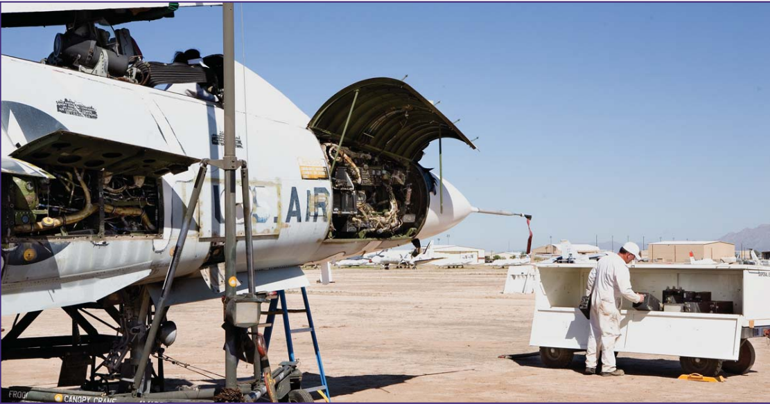
Disposal team member, Mr. Phil Kovaric, places aircraft components removed from a F-101 "Voodoo" in a trailered container designed to transfer and securely store items prior to final demilitarization.
