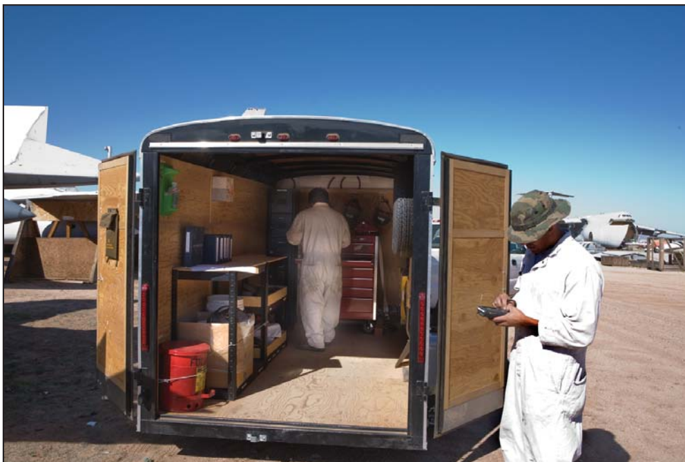
Mr. Manny Guaman and Mr. Chris Hodgson (r) retrieve specialized tools from one of five portable trailers housing composite tool kits (CTKs) specifically designed for aircraft demilitarization activities.
