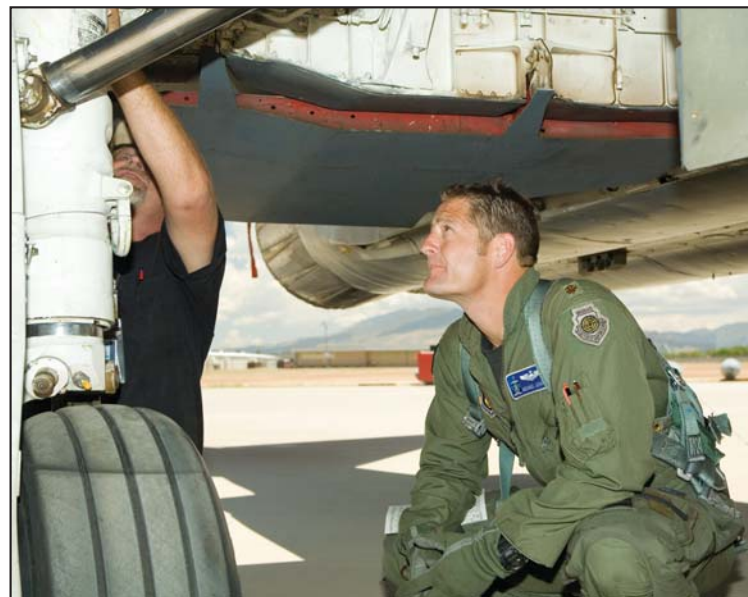
Aircraft worker, Mr. Gary Snipes (l) and Major Leach or “Shot” discuss a main landing gear strut during a pre-flight inspection on a QF-4 (drone) aircraft.
