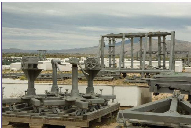
Almost 320,000 pieces of production tooling from the assembly lines of B-1B, EA-6B, C-135, B-52, B-2 and other military aircraft are stored at 309 AMARG. Pictured above is an aircraft assembly jig.
