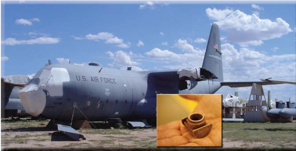
One of the many C-130 aircraft currently stored at 309 AMARG serving as a critical parts resource. In March, more than 500 barrel nuts were removed from the desert and shipped to the customer on the battlefield. Actual C-130 aircraft barrel nut shown in inset photo.
