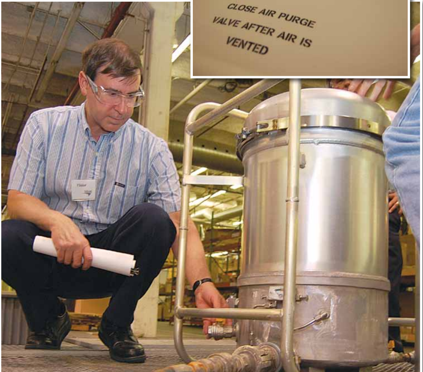
David Peterson, Defense Contract Management Agency Denver quality assurance specialist, inspects a 50 gallon-per-minute fuel filter assembly along with team members. This product helps protect and extend the life of military equipment — mainly aviation applications.
