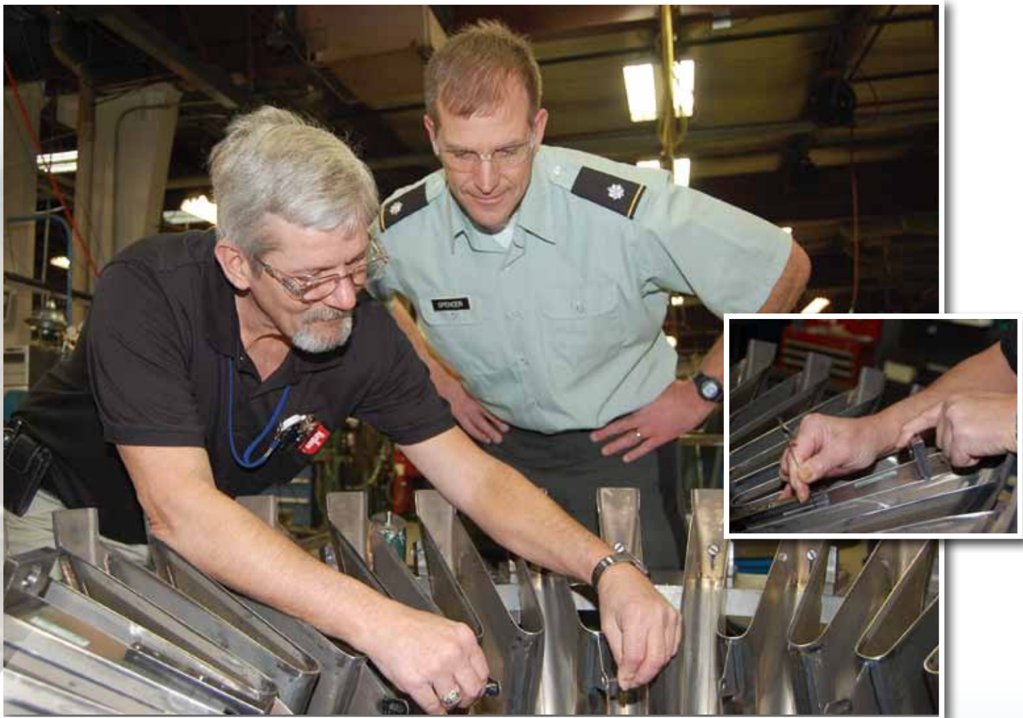
Gary Haton (left), Defense Contract Management Agency Indianapolis quality assurance specialist, demonstrates to Army Lt. Col. Todd Spencer, DCMA Indianapolis commander, how he checks the slot width of an aircraft engine part using go, no-go gauge pins.
