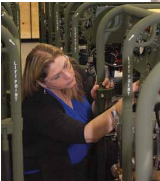
During final inspection, Defense Contract Management Agency Dayton quality assurance specialist Jennifer Sheriff checks to ensure the proper assembly and functionality of a M26 joint service transportable decontamination system — small scale. (Photos by Jo Adail Stephenson, DCMA Public Affairs)
