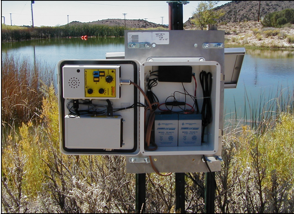
Figure 6-12. Passive acoustic monitoring system at Camp 17 Pond
