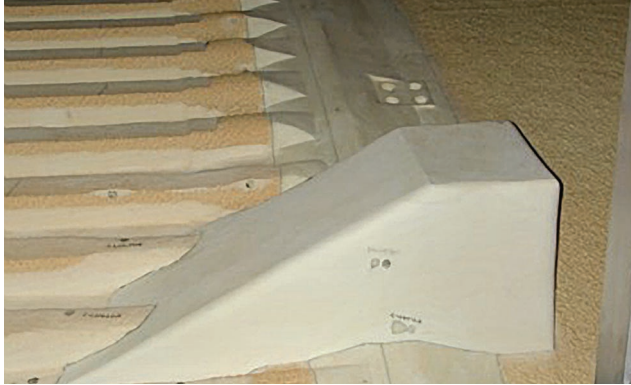
Figure 3.2-1-2. ET forward bipod ramp (foam).
