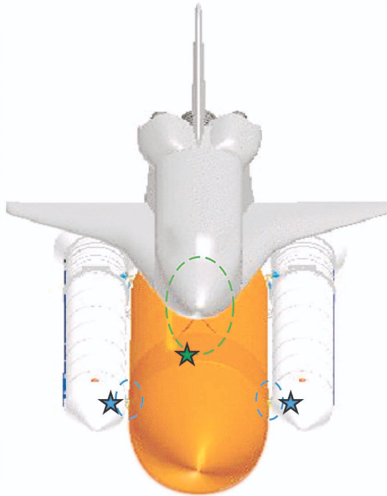
Figure 3.4-3-1. ET flight cameras (STS-114 configuration).
