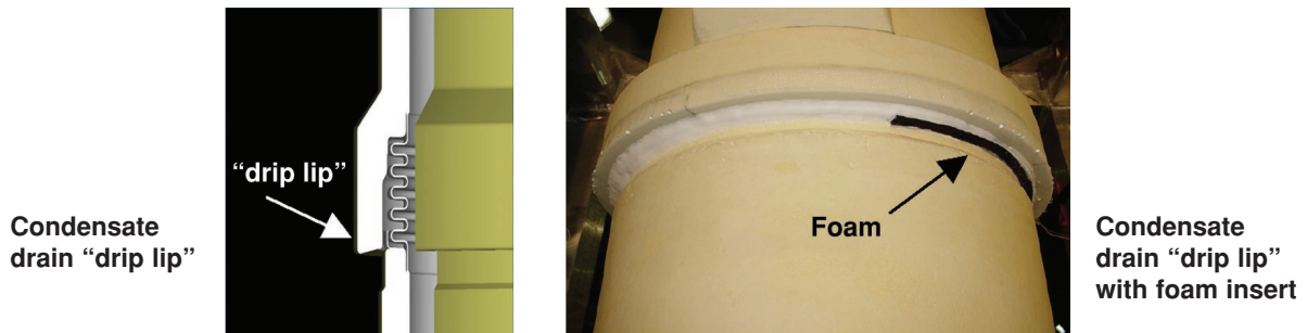
Figure 3.2-1-11. LO 2 feedline bellows 'drip lip' with foam insert.
