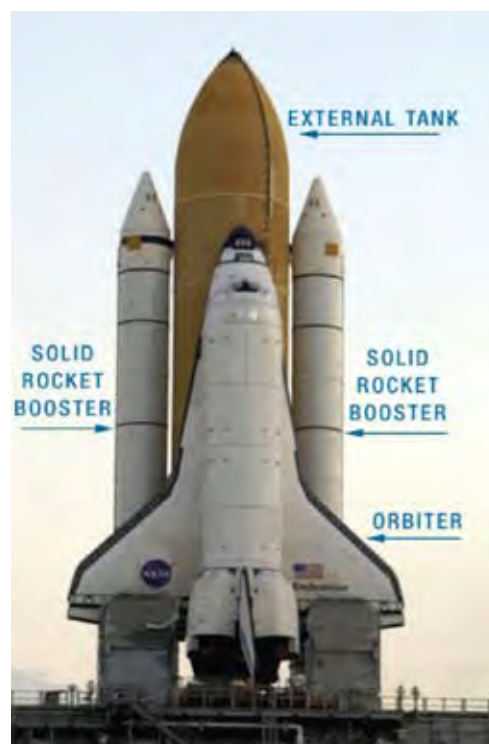
Figure 4.1.1-1. The principal components of the Space Shuttle. Source: NASA
