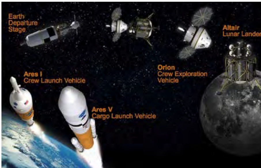
Figure 4.3-1. The major elements of the Constellation transportation architecture showing sequence of operation. Source: NASA
