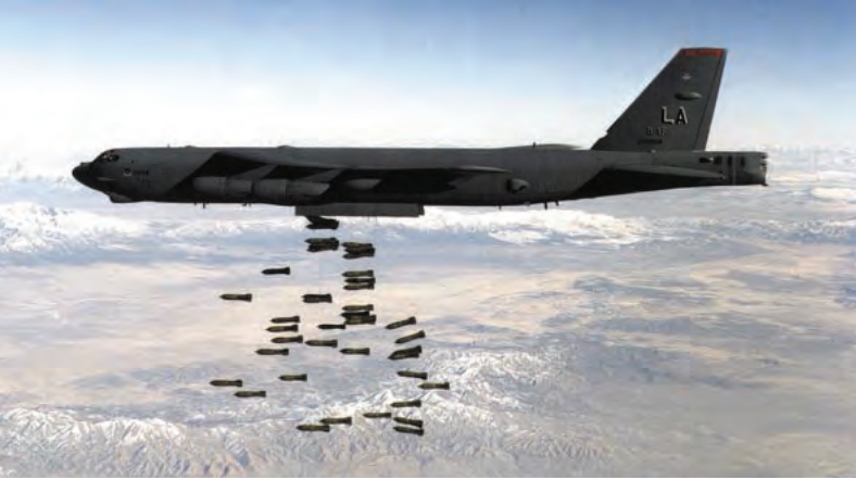
Many aerospace systems, like the B-52, are on the path to an operational life of 50-75 years though their original design life was only 20-30 years.
