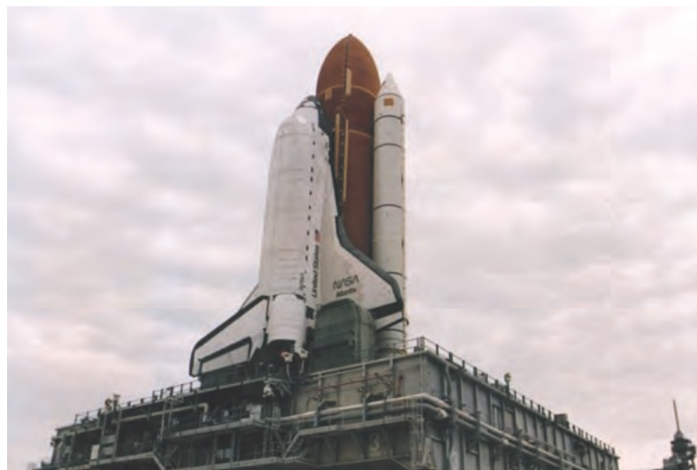
The Crawler/Transporters, used to move the assembled Space Shuttle system to the launch pad, are over 30 years old.
