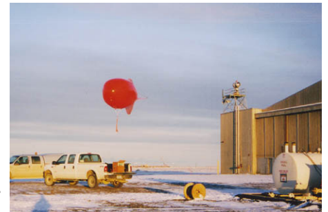
An instrumented tethered balloon is one way to gather atmospheric data. With Recovery Act funding, the ARM program can lease time on unmanned aerial vehicles.
