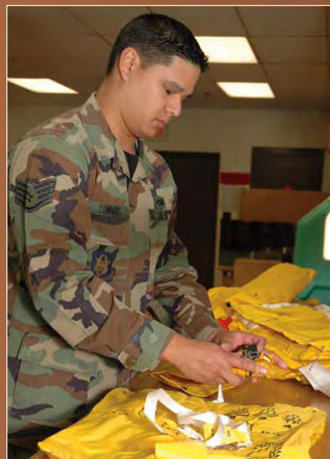
Fabric worker, Staff Sgt. Steve Connors, repacks an adult/child floatation device after completing routine inspection of a 128-pack of the devices. These life preservers are stored on the wing's aircraft in the event passengers are onboard.
