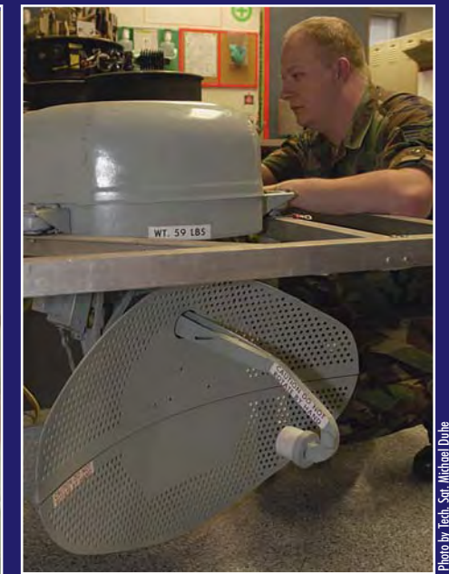
Staff Sgt. Anthony Hinkel checks the connections on a C-130H weather radar antenna. The radar systems have been a workhorse for Hurricane Hunter missions and are brought in to the Comm-Nav shop for repair and checked for operability.
