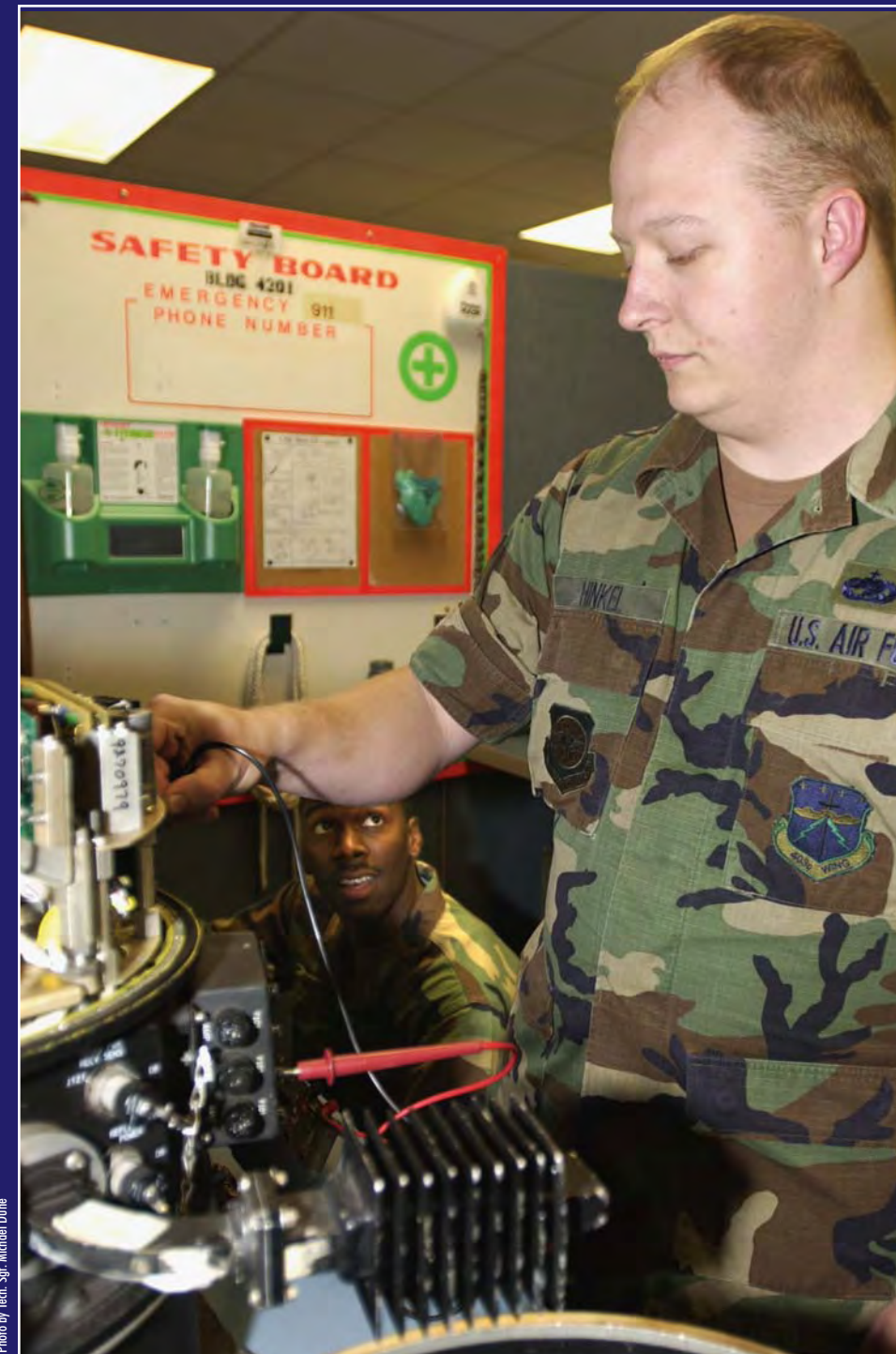
Staff Sgt. Anthony Hinkel (foreground) checks a fuse on a C-130H radar as Tech Sgt. Ronald Martin monitors the power settings. Both Airmen are integrated systems technicians with the 403rd Avionics Flight's Comm-Nav shop. The radar systems are brought in to the Comm-Nav shop for repair and checked for operability on a regular basis.
