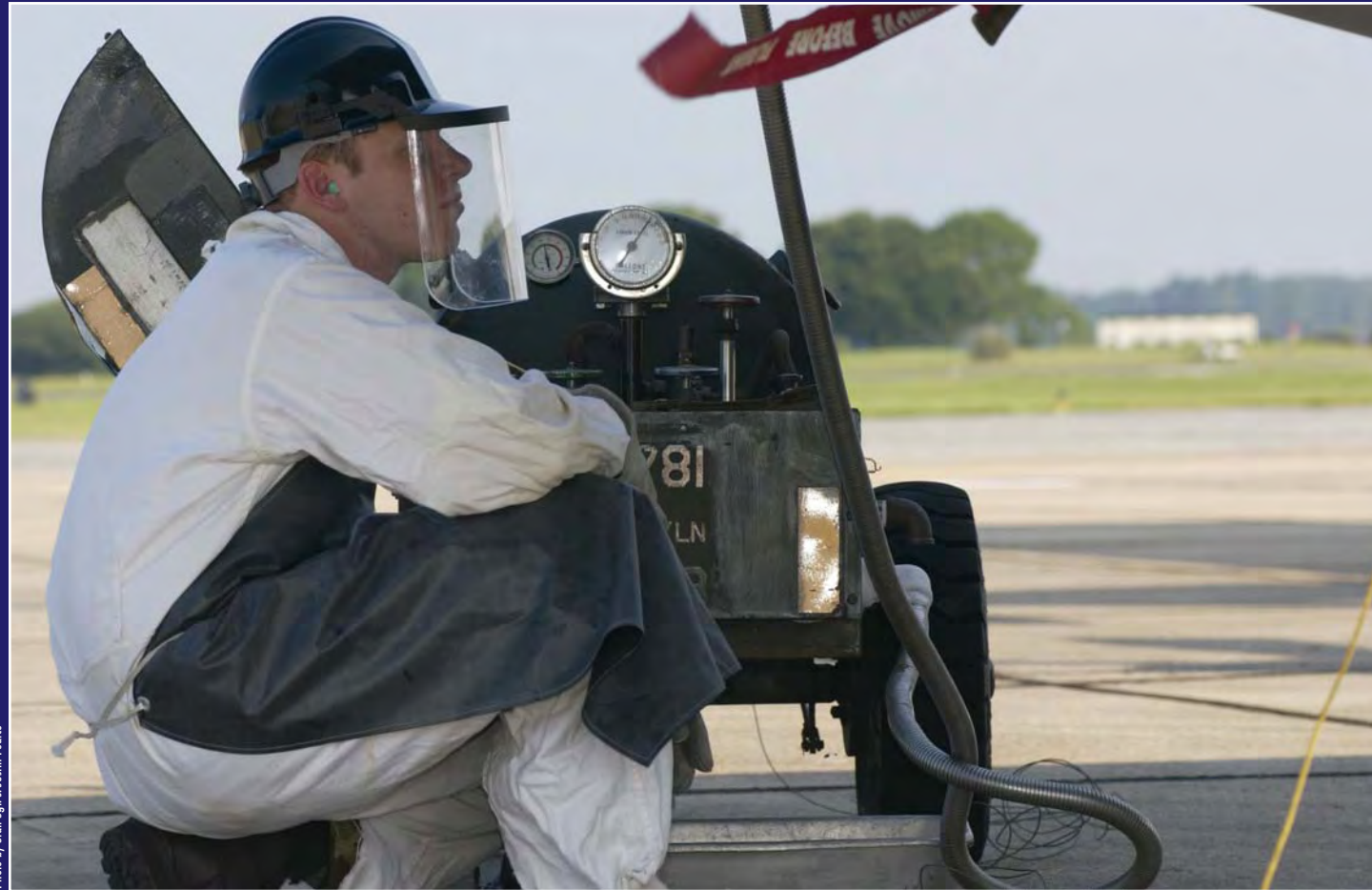
On a hot UTA Sunday in July, Senior Airman Michael Staten, a crew chief with the 403rd Aircraft Maintenance Squadron, pumps liquid oxygen into a Hercules C-130H. The liquid oxygen, or LOX, is stored on board for aircrew to use in emergencies and for high altitude flying when the crew compartments cannot be pressurized. Read more about it on Page 14.
