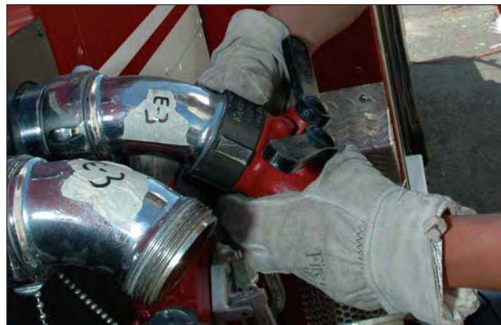
A firefighter with the 403rd CES Fire Department, attaches a hose to the discharge outlet of a fire truck.
