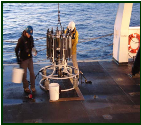
Water collection from Niskin bottles
