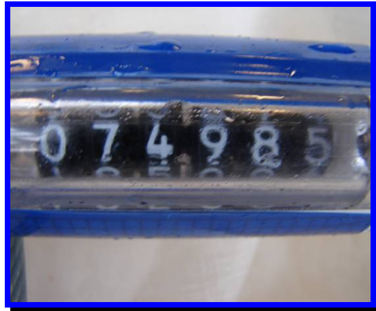
Mechanical counter in flowmeter
