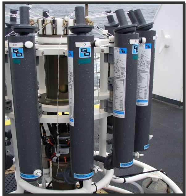
Open Niskin bottles on CTD platform
