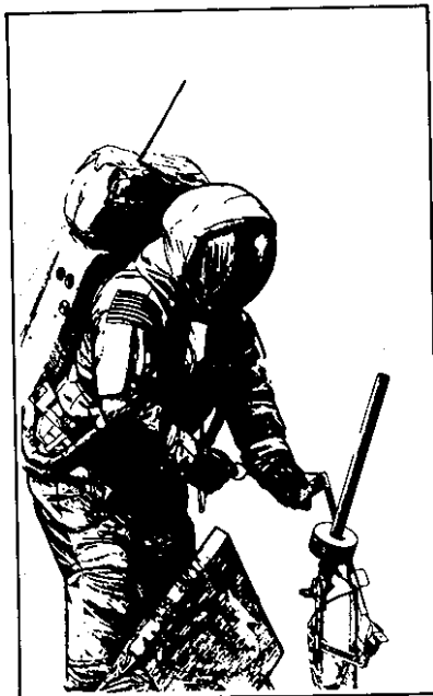
Alignment Of Passive Seismometer
