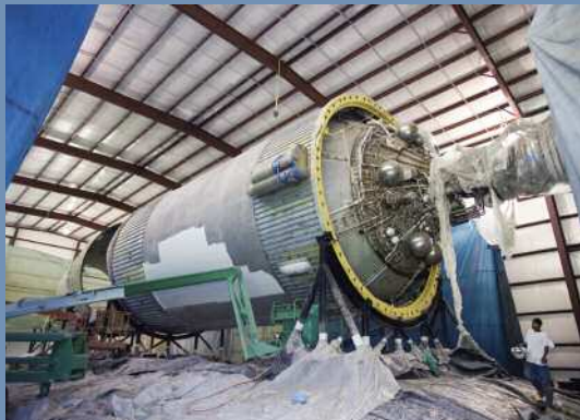
Multiple layers of the rocket’s exterior paint were removed using ultra-high pressure water jets.
