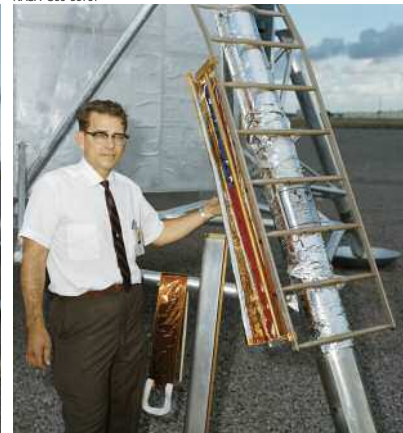
On a mock-up of the Lunar Module, David McCraw demonstrates the deployment sequence of the flag, following step-by-step procedures created for the astronauts. The entire flag unit fit into a three-foot protective heat shroud, stored on the side of the descent stage ladder.
