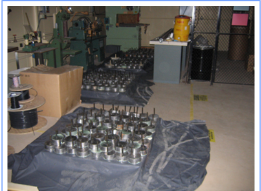
Lead plugs used for shielding in instrument and power cable penetrations to hot cell - reuse as shielding blocks at another DOE site.
