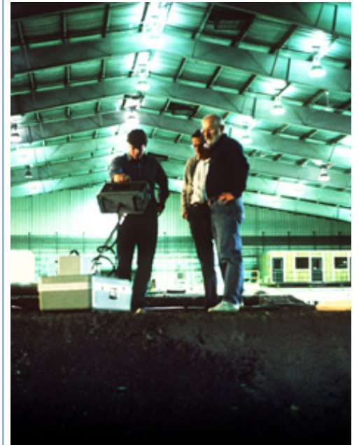
Duane Gardner (GPR operator, left) conducts a coal measurement experiment with GPR for representatives of U.S. Bureau of Mines (standing on mound of coal).
