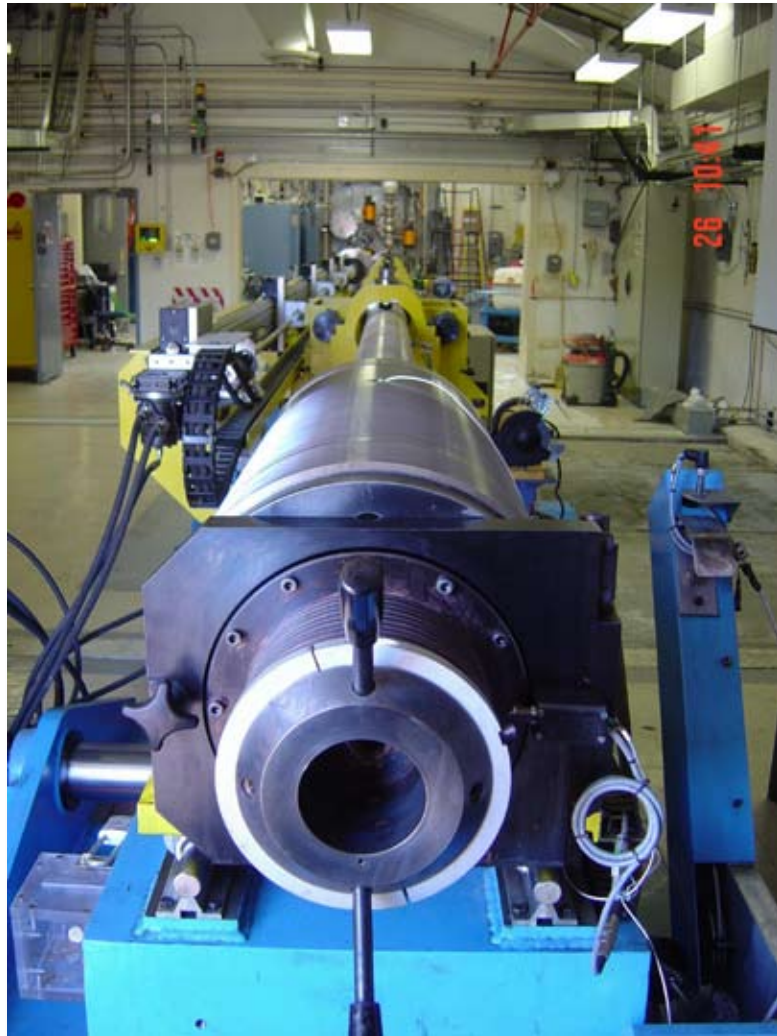
This perspective shows the breech end of the gas gun, down the barrel, to the secondary containment chamber. JASPER provides a way to generate and then measure data that is crucial to certify the safety of the stockpile.
